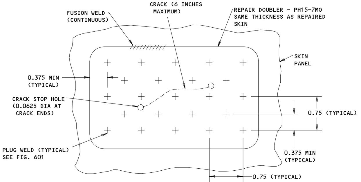
**REPAIR OF 2- TO 6-INCH CRACK IN SOLID SKIN**
