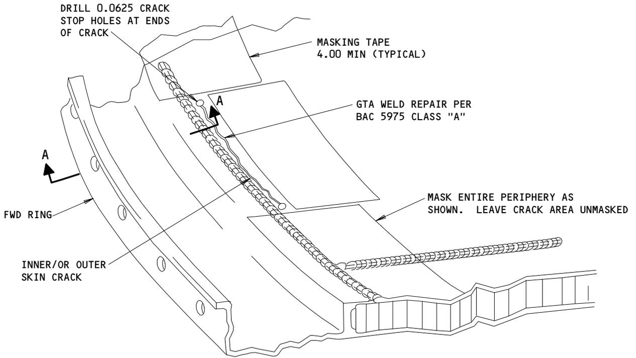
0.125 DIA PURGE GAS HOLE NEAR CENTER OF REPAIR, WELD SHUT WHEN REPAIR IS COMPLETE
