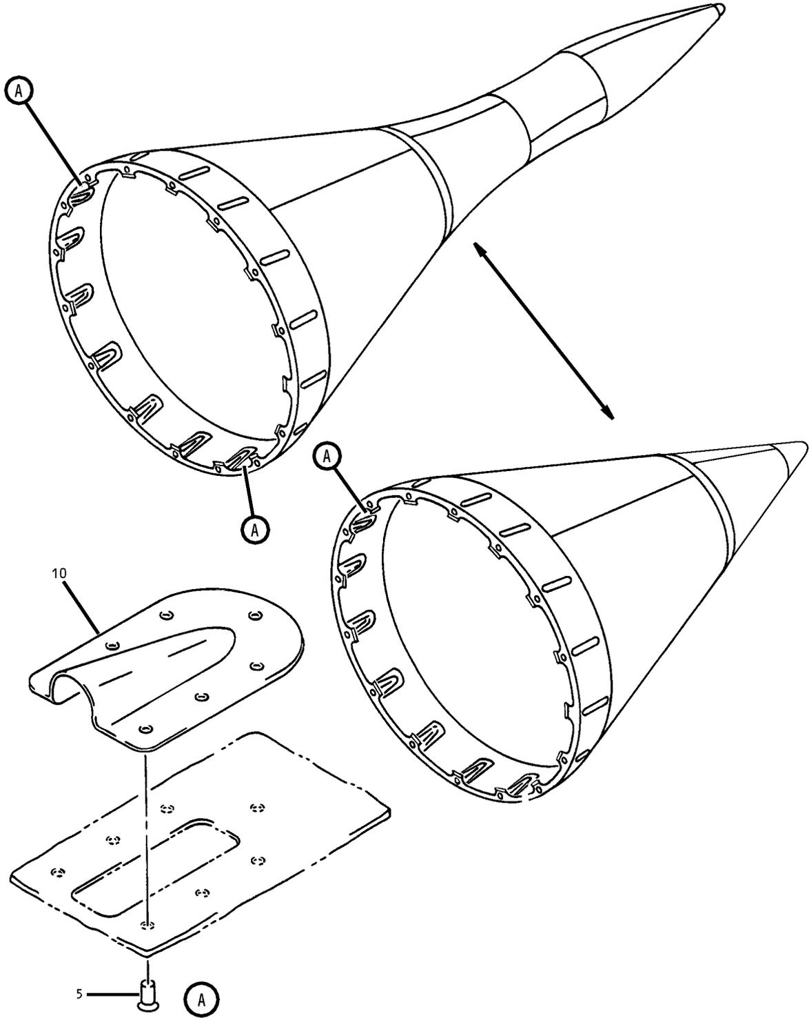
Turbine Exhaust System Plug Assembly
