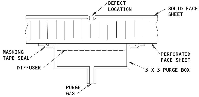
PURGE SETUP FOR REPAIR
