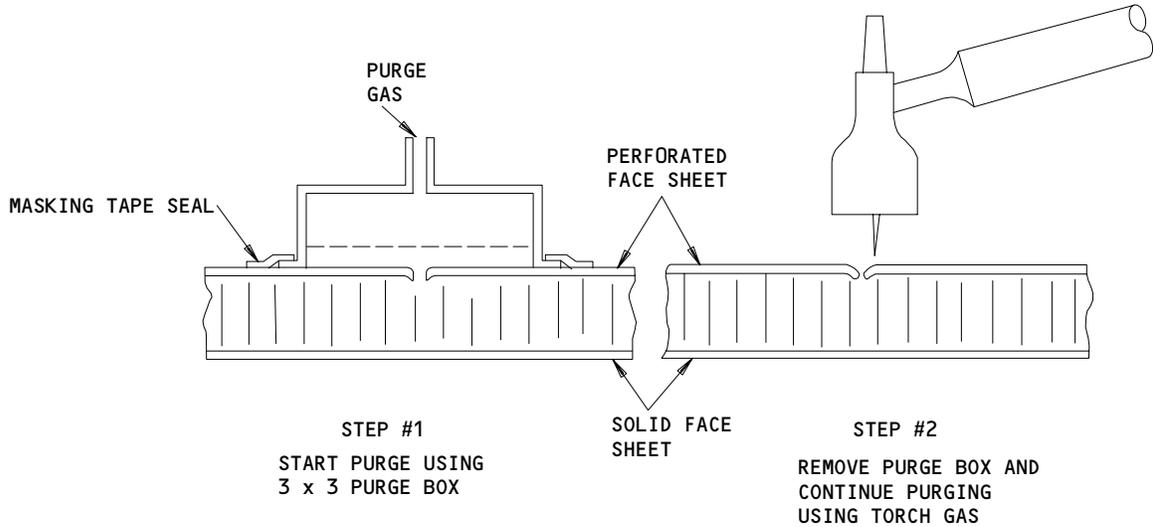
PURGE SETUP FOR REPAIR WELD
